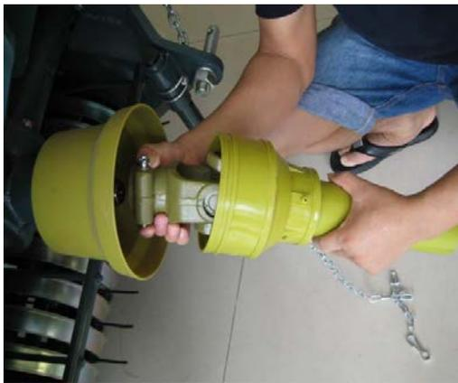
Fig. 13. The universal shaft connected to the tractor's PTO.
