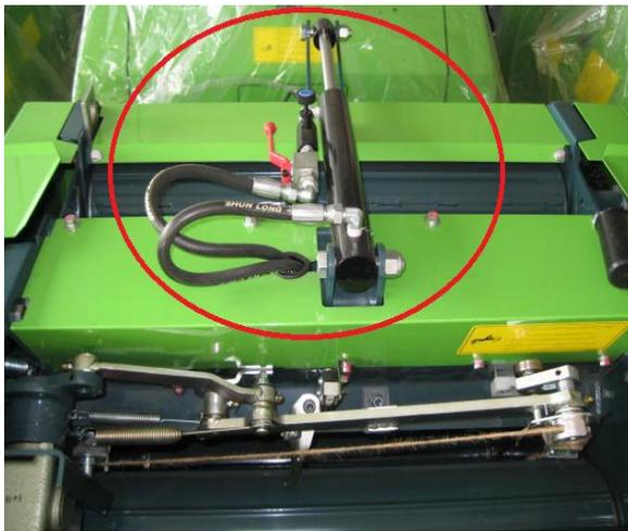
The hydraulic piston (encircled in red) enables unloading of baled straw when baling is completed and tying is done.
