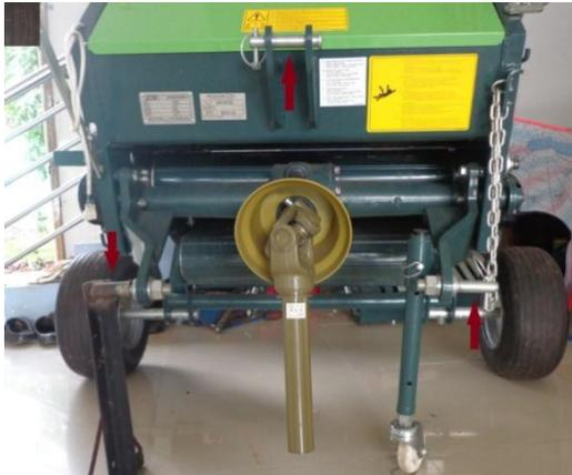
Fig. 12. Three-point linkage for connecting the baler to the tractor.
