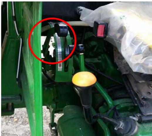
Fig.19. Hydraulic lever of the tractor.
