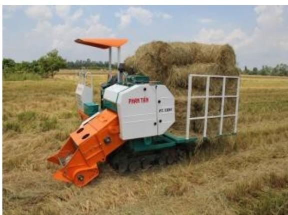
Fig. 5. Self-propelled baler.
