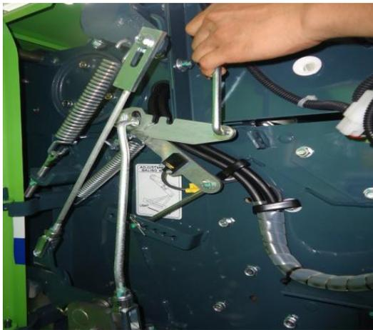
Fig. 18. Adjusting bale compaction.
