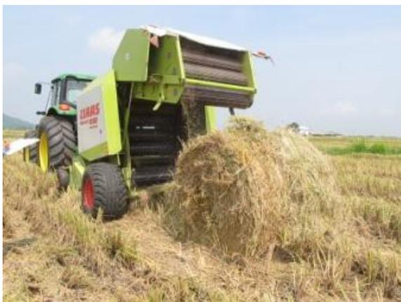
Fig. 3. Large-scale roller baler - (500 kg/bale).
