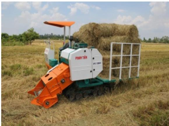
Figure 5c. Self-propelled baler.
