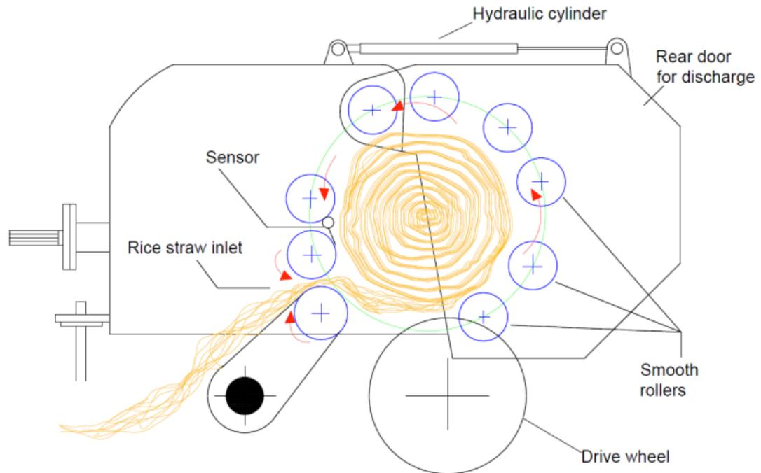
**Figure 4a. Roller-type straw baler (right side view).**
