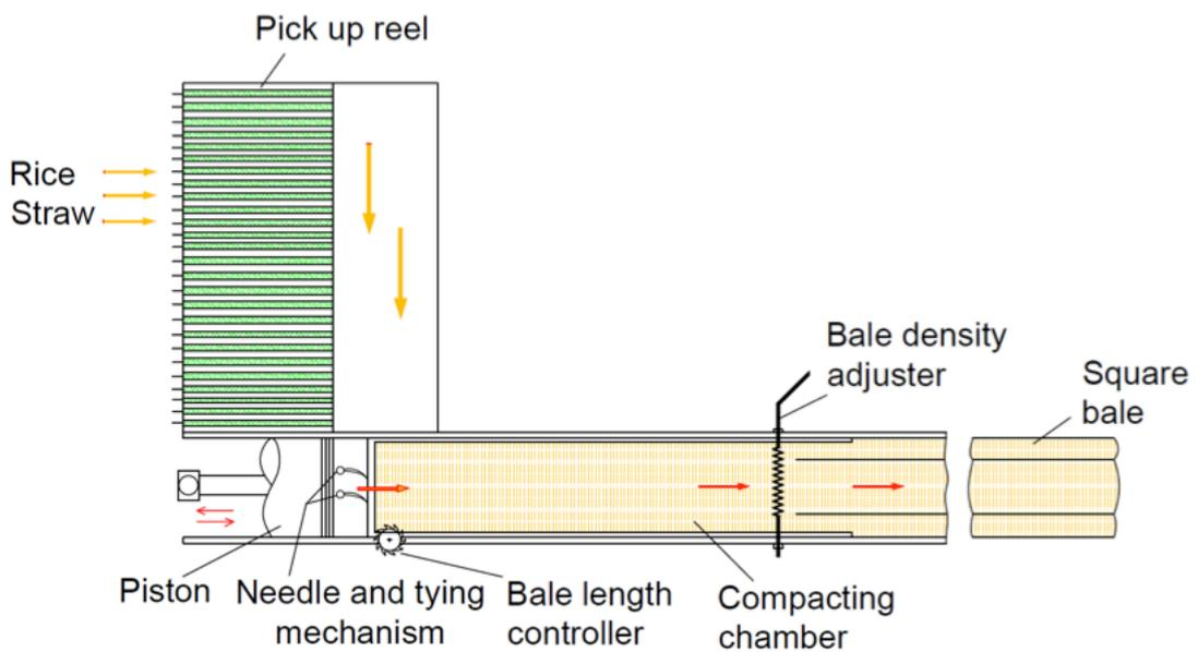
**Figure 4b. Piston-type rice straw baler (top view).**
