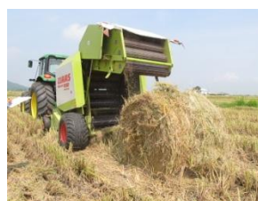
Figure 3. Roller baler: straw bales (500 kg/bale) left in the field, need heavy vehicles for handling; cannot work in wet field.
