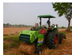
Figure 4. Roller baler: straw bales (13 kg/bale) left in the field, need vehicles for handling; cannot work in wet field.
