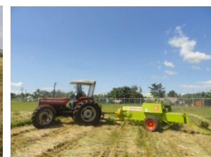
Figure 6. Square baler: straw bales (18 kg/bale) left in the field, need vehicles for handling; cannot work in wet field.
