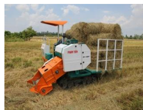
Figure 5. Self-propelled baler: combines baling and transporting rice straw to the bund; workable in wet field.
